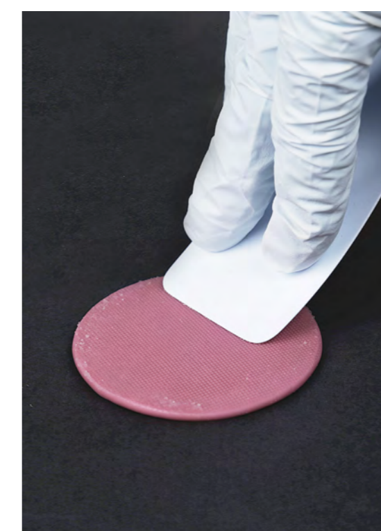
Fig. 4: Introduction of adhesive gel with a spatula and scraper
