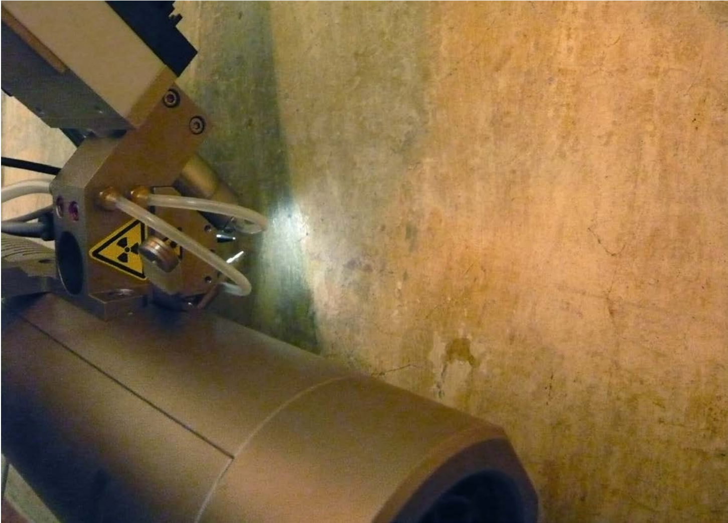
X-Ray microfluorescence measurement, detail of frescoes, chapel, Charterhouse, Villeneuve-lès-Avignon (France), 1355; Photo: 2011, CICRP (Jean-Marc Vallet)
