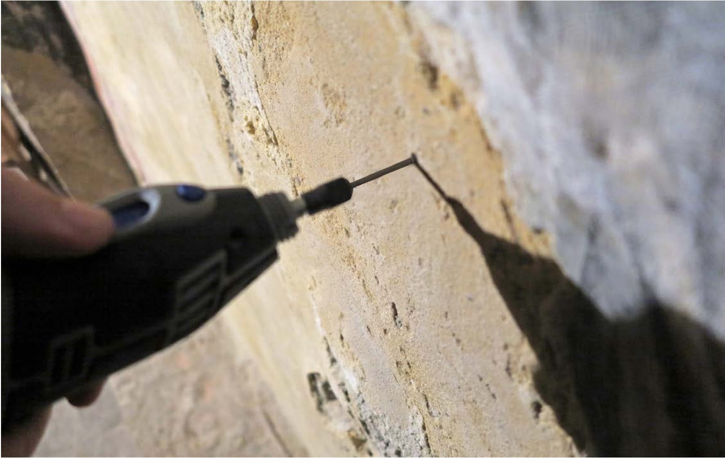
Drill core sampling of a restoration render, Chapel of Notre Dame d'Entrevignes, Sigale (France), 16th century; Photo: 2013, CICRP (Jean-Marc Vallet)
