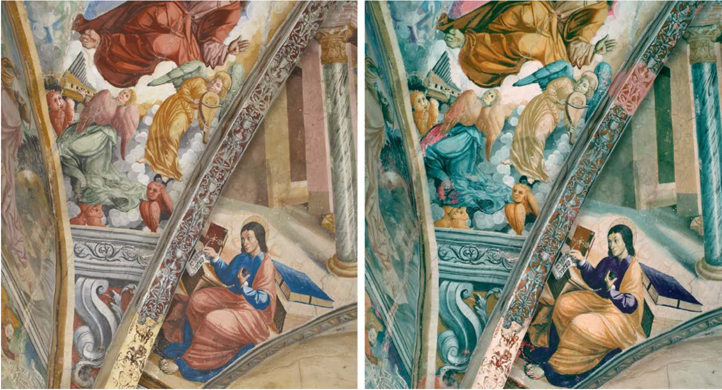
Viewing of restored area in direct light (left) and IR false colour (right), Chapel of Notre Dame d'Entrevignes, Sigale (France), 16th century; Photo: 2013, CICRP (Odile Guillon)
