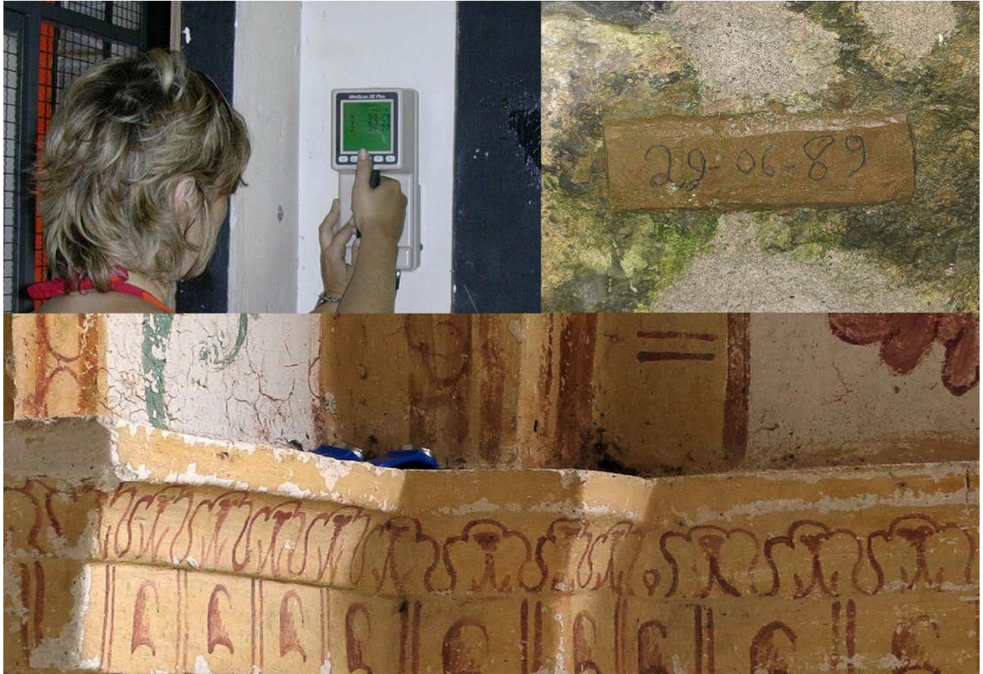
Collecting colorimetric data (top, left), crack monitor to observe deformations (top, right), Villa E-1027, Roquebrune- Cap Martin (France), 20th century and climate data logger (bottom), Chapel of Notre-Dame des Fontaines, La Brigue (France), 15th century; Photos: 2007/2014, CICRP (Jean-Marc Vallet)
