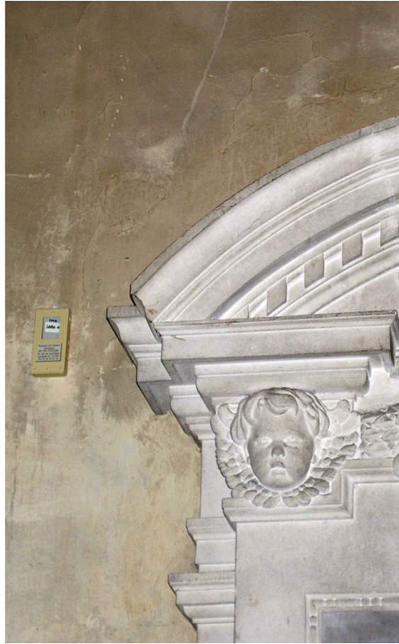
Relative humidity and temperature monitoring, Chapel of Saint Lazare, Aix en Provence Cathedral (France), 12-16th century; Photos: 2000-2004, CICRP (Jean-Marc Vallet)
