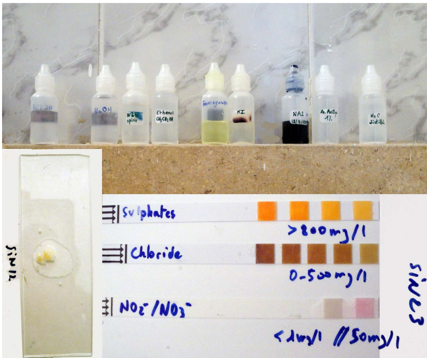
Chemical reagents (top), microchemical test (bottom, left), salt testing using chemical strips (bottom, right) on samples from Coptic wall paintings in a cave at the site of Hammâm Faraûn Sinaï (Egypt); Photos: 2010, CICRP (Jean-Marc Vallet)
