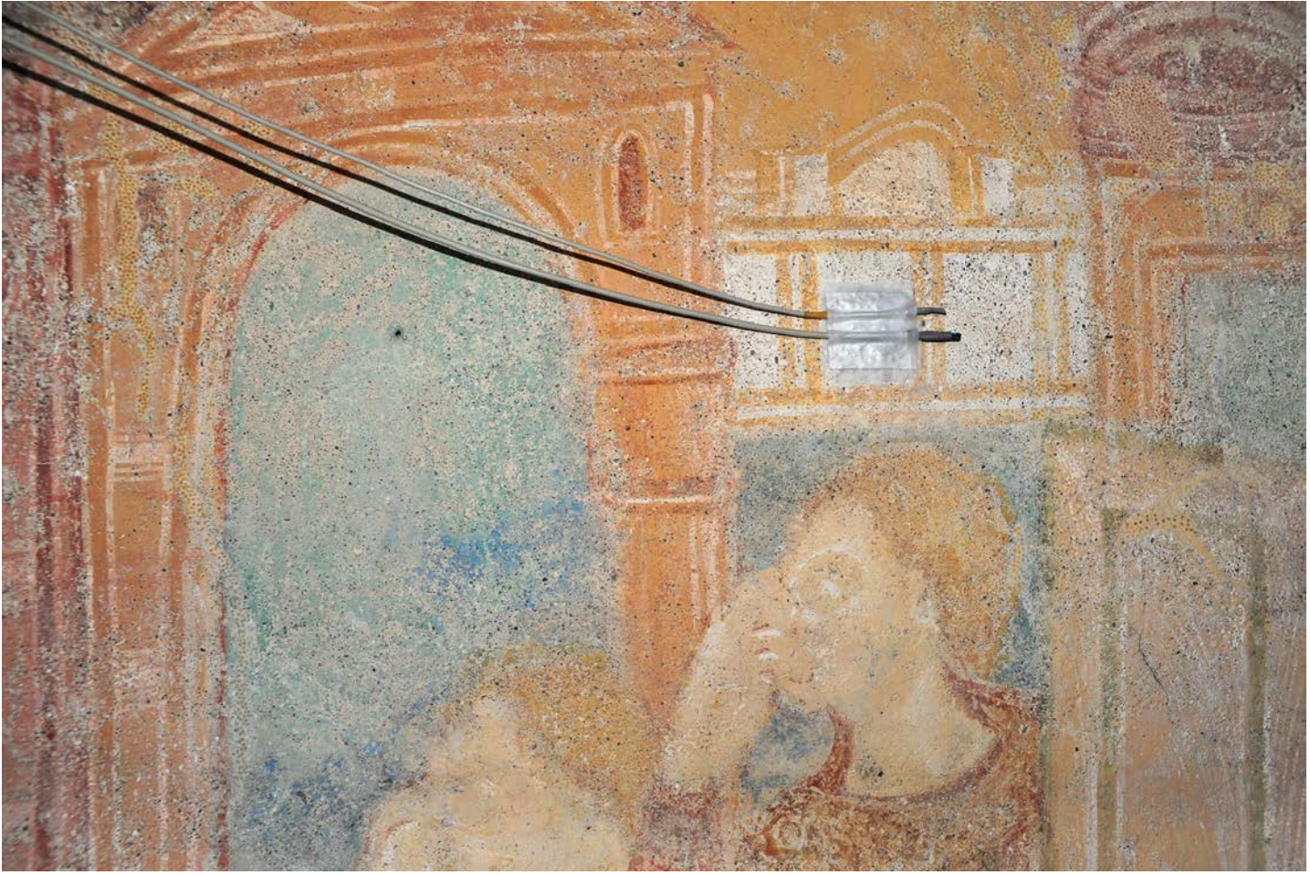
Sensors for environmental monitoring temporarily fixed with binder which sublimates (cyclododecane), St. Georg, Reichenau-Oberzell (Germany), 10th century; Photo: 2014, RPS (Dörthe Jakobs)
