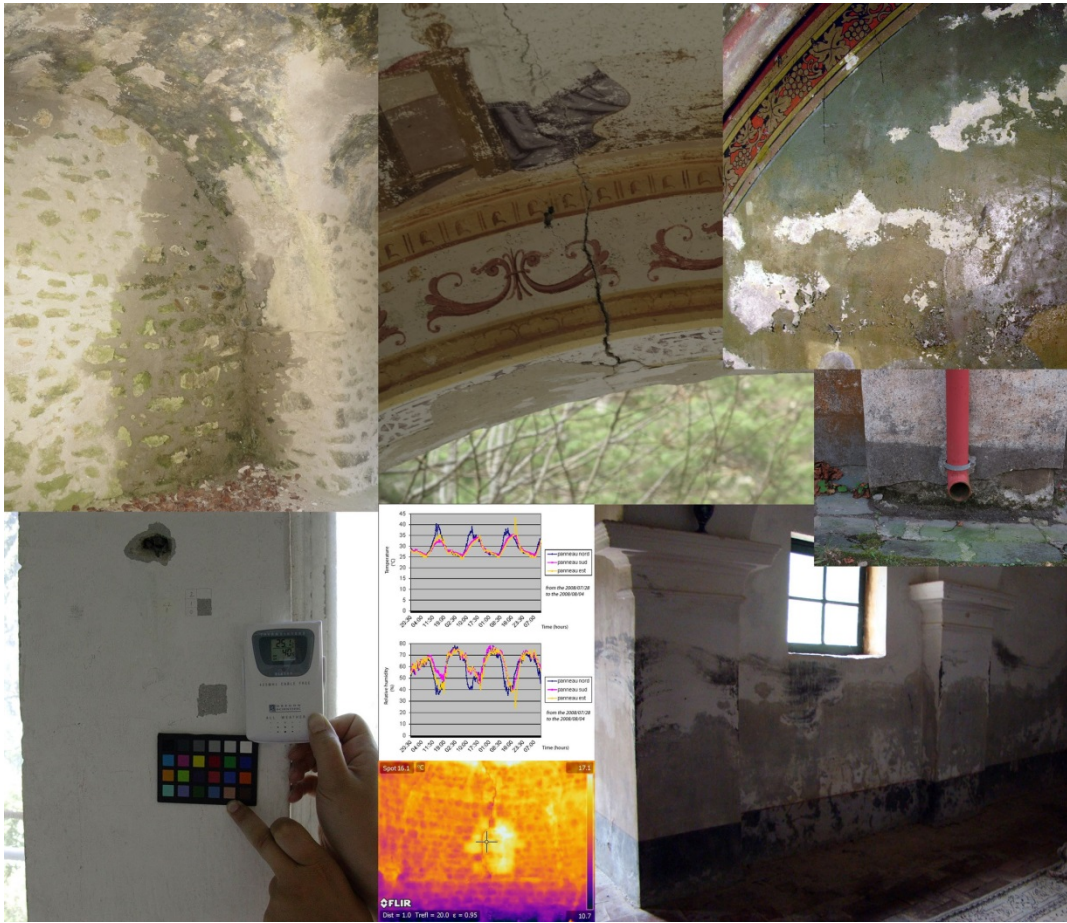
Monitoring including relative humidity and temperature measurements (bottom, left and centre) and observations including passive IR thermography (bottom, centre) relative to environmental issues; Photos: CICRP (Jean-Marc Vallet)
